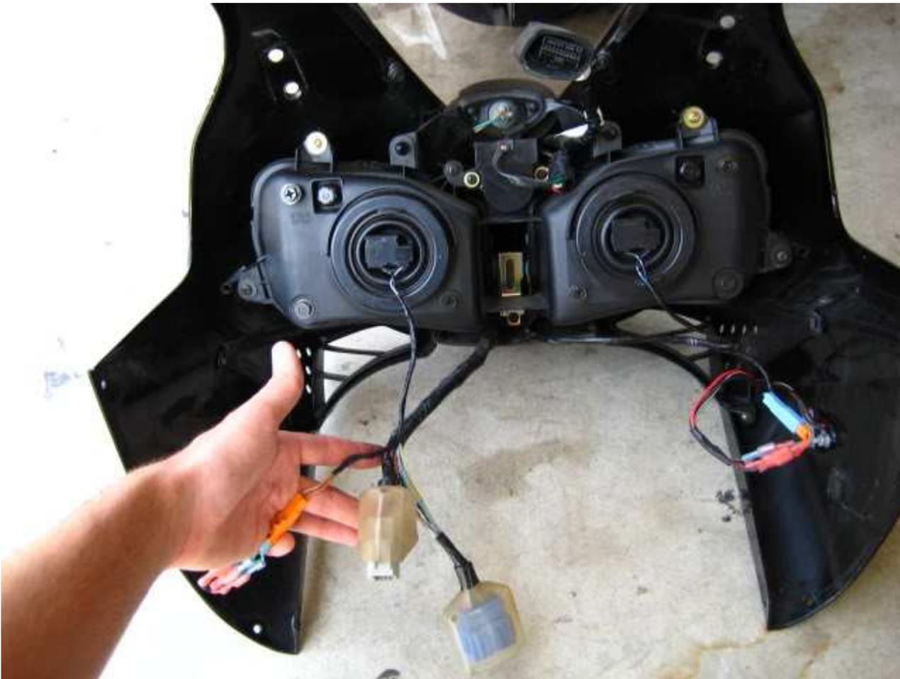
**Step 5** - Now let's separate our fairing from our headlight assembly. The 5 screws circled in red need to be removed as well as a hidden [circled in yellow] Philips screw underneath the headlight relay.
