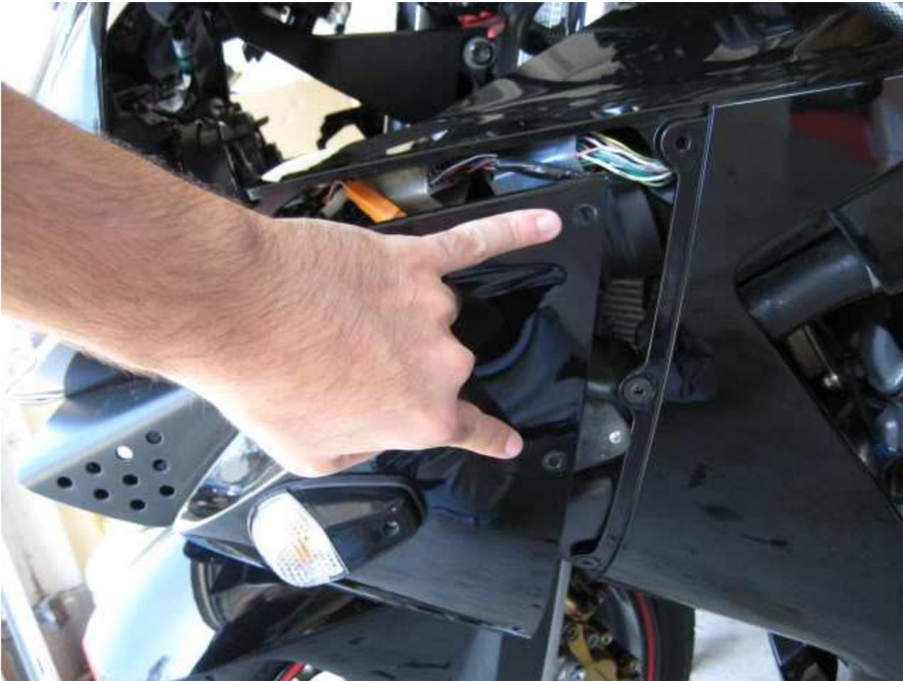
**Step 2** - Make sure you've removed the 2 inner lower fairing clips on both the left and right sides. And the one clip on the center and underside of the nose.
