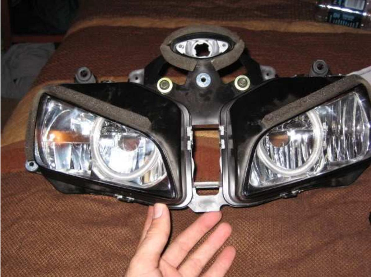
**Step 8** – Wiring the rings is required. The provided inverter needs to sit outside the headlight, Velcro or twist ties to prevent too much dangling or shock.
