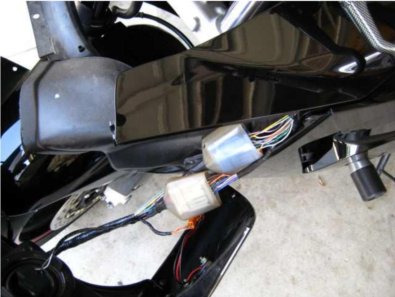
**Step 4** - Now that we have removed our fairing lets first start with finding a clean and stable surface to work with. We have a towel and blanket onto a table which works great. Remove your bulbs and the rubber gasket/covers from them first. Here's a naked layout of the upper fairing and headlight assembly together.
