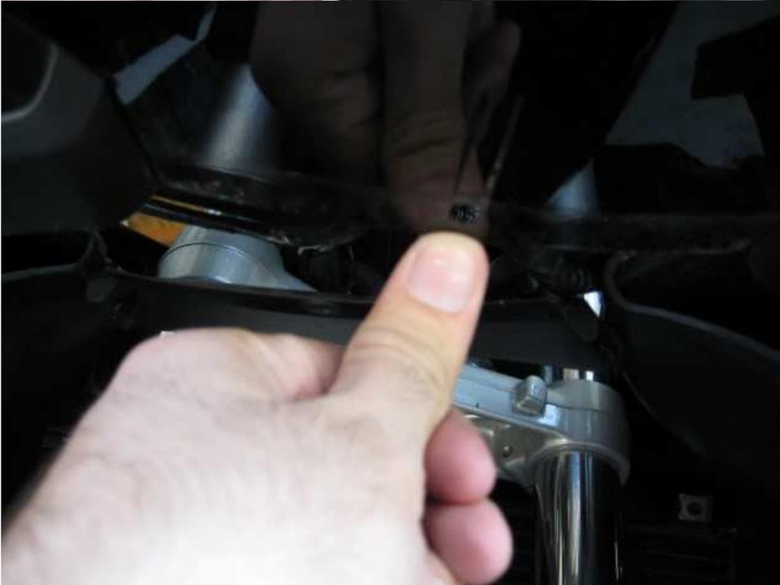
**Step 3** - You will notice that the fairing is now basically dangling and being held on by nothing more than 3 clips. 1 clip going to your cluster/speedo which is black. A grey plug and a blue which [connect](#) to the rest of the harness and head further down toward the rear of the bike.
