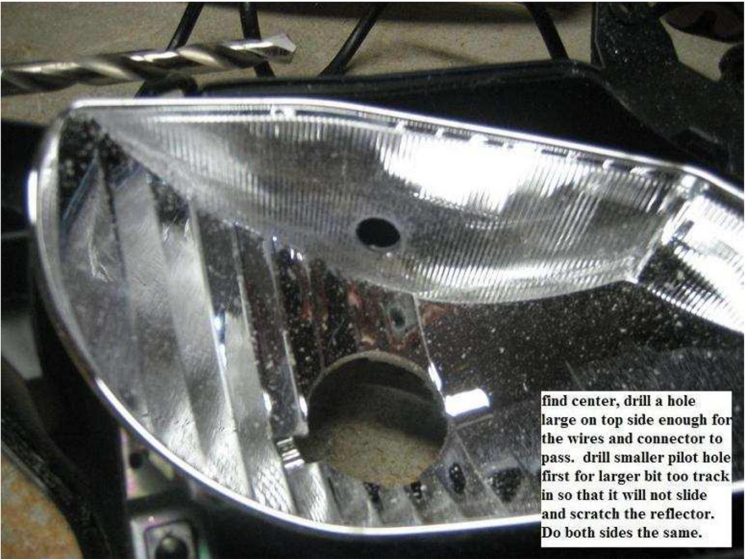
find center, drill a hole large on top side enough for the wires and connector to pass. drill smaller pilot hole first for larger bit too track in so that it will not slide and scratch the reflector. Do both sides the same.
