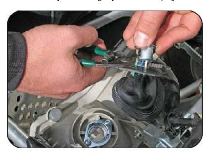
Once cut, you can decide if you want to wire the HID it to your low beam wire or your high beam wire. This will make a difference on how the switch works. We generally recommend having your HID kit come on after the ATV is started. This way there is no electrical dips while the engine is cranking.
