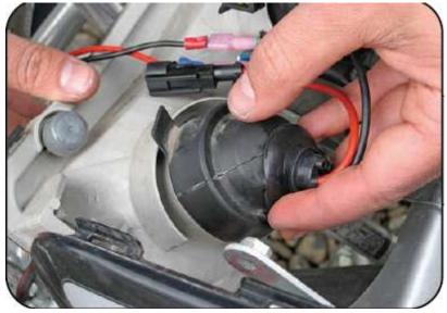
12. Connect the two round connecters from the bulb to the ballast
