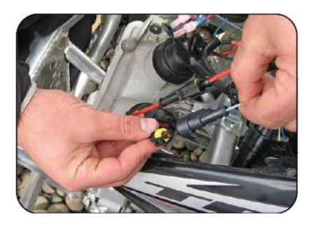
13. Plug the oval connector leading from the ATV wiring to the ballast.
