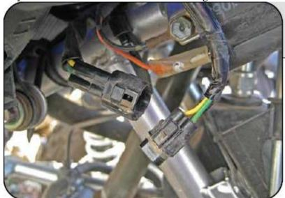
6. Locate the provided two wires and white plastic adapter plug. You will insert the two ends into the correct spot for Ground/Low beam of the white plug. This plug then will plug into your factory harness.
