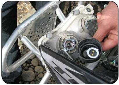
4. Remove the factory H6m bulb
