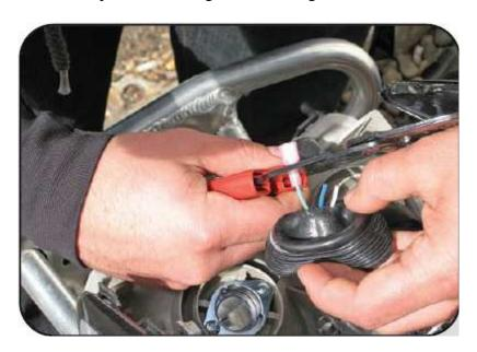
Wire the ground and low beam positive wire directly to the end of the provided wire. You can use pliers and electrical tape to make a good connection.
